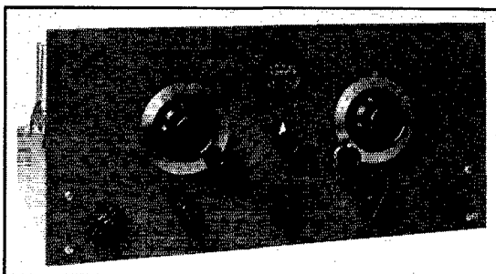
SEPARATE VERNIER TUNING CONTROLS ARE PROVIDED FOR THE SELF-CONTROLLED OSCILLATOR AND THE 807 OUTPUT STAGE
